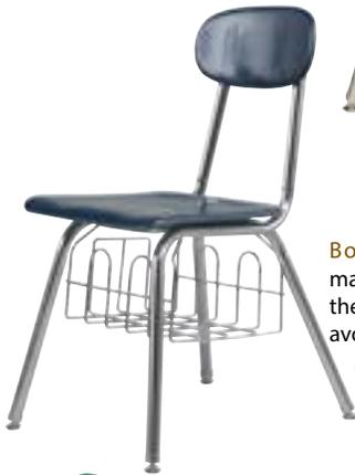
**Bookrack:** 12-1/2" x 11" x 6" made of 1/4" steel rod and welded to the frame at four points. Designed to avoid use as a footrest.
